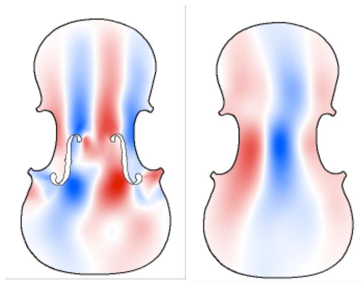
Here is the same B1+ mode shape but showing the cross-grain bending. The two colours indicate whether the bending is concave or convex and the intensity of colour the radius of curvature. A small radius is tight bending and will have strong colour whereas a flat surface has infinite radius and would be white.
