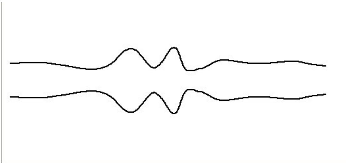
Certainly part of the explanation is the weakening of the plate by the f holes particularly at the eyes. This allows the island to twist more than the areas above and below the holes. Another factor may be the compression along the grain due to the string tension. A modal analysis of a violin with the strings tuned down (just enough tension to keep the bridge in place) appears to have less complicated long-grain bending than the same violin tuned to pitch.
