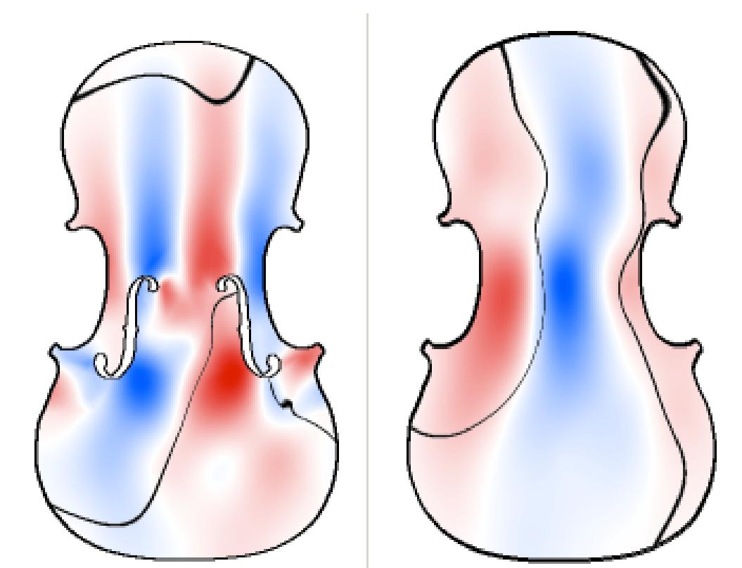
While there is a strong correspondence between the displacement and the bending for the back this is not so for the front. We would see more extreme examples in other modes. Modes store their energy alternately in the motion of the mass and in the spring energy of bending areas. If we could do the same for the in-plane motion we would see that energy is also stored in lateral distortion and motion. The Polytec 3D laser plots clearly show that in-plane motion is frequently significant.
