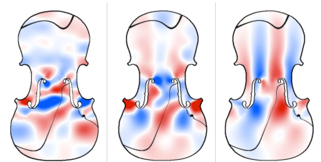
The complication in the long-grain bending is perhaps surprising. Below are both phases of a displacement slice taken approximately along the bass bar. (Tail block to the left and neck to the right)
