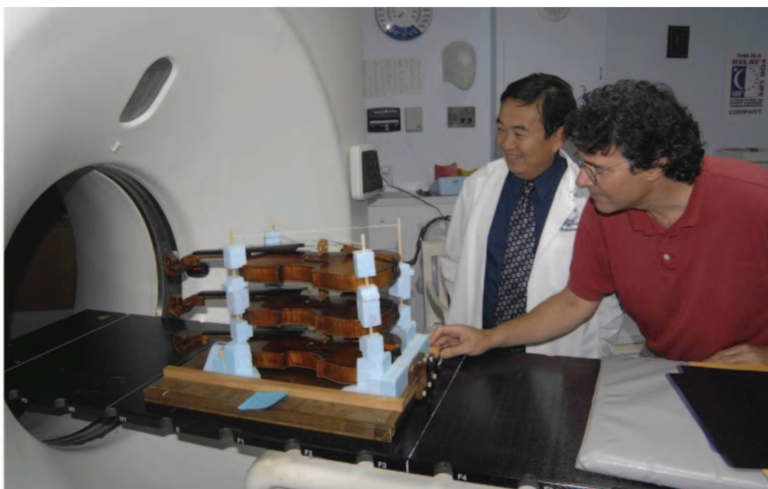
Figure 8. The Old Italian violins were stacked three high (bottom to top: the Titian, the Plowden, and the Willemotte) for the CT scan measurements. The scans were performed by Dr. Claudio Sibata, head of Medical Physics staff at the Leo Jenkins Cancer Center, with the assistance of Sam Zygmuntowicz.
