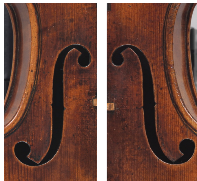
The f-holes have confidently cut, upright stems, with wide, well-scooped lower wings
