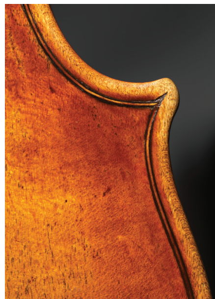
Right Conversely, the strips in the lower bass-side corner do not exactly meet in a mitre
