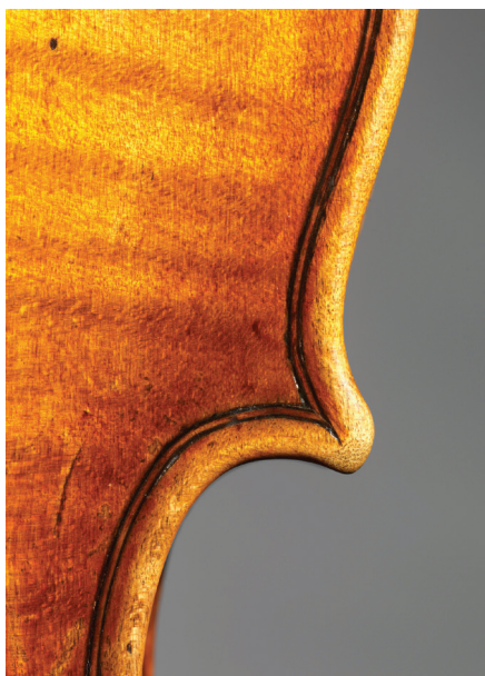
Left The purfling in the upper bass-side corner ends in a classic bee-sting
