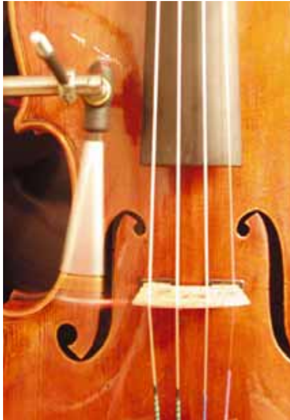
ABOVE hitting the side of the bridge with a small hammer is a simple way to excite the violin across a broad frequency range
