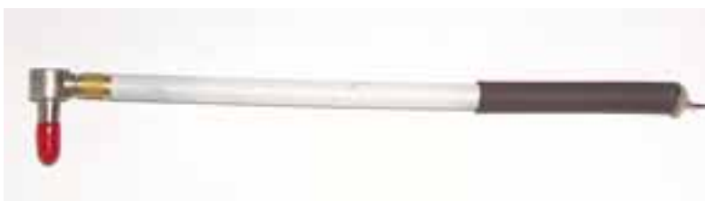
ABOVE the PCB Piezotronics impact hammer has a sensor in the tip which can be calibrated to allow accurate measurements
